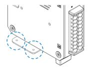
4) Similarly, install the Alarm Module on the last part and fix with screws (Recommended tightening torque: 4kgf/cm). Tighten the lower part after first tightening the upper part.
