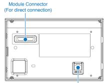
Monitor In connector (For connecting cable)
