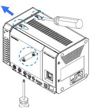
3) Slide the Amplifier Module parallel to the GL7000 and connect the connector.
