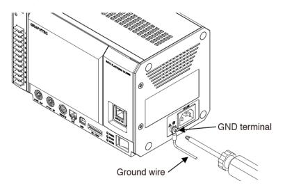
\*In order to prevent an electric shock and a fire, please be sure to ground using a GND terminal.For grounding, use a ground wire with a diameter of at least 0.75 mm2.
